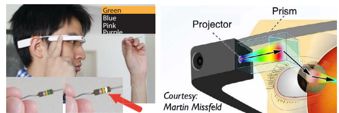
Figure 4: Left: colorblind user wearing Glass; in the detail Chroma’s menu and the results of the Green Highlighting on a resistor. Right: Glass’s semi-transparent prism acting as display, and micro-projector casting the image on the prism. The projected image is reflected on the user’s retina.
